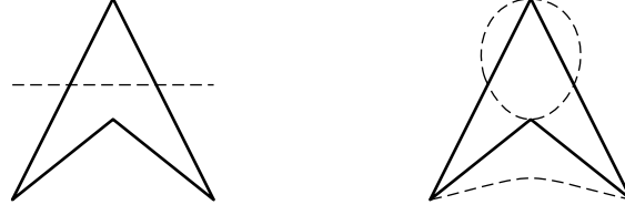
Figure 2.3. Zero level set (dashed) of the denominator W for the Wachspress (left) and the discrete harmonic (right) coordinates with respect to a concave polygon. In both cases, the zero level curves cross the polygon's interior and hence the coordinates are not well-defined at the corresponding points.
